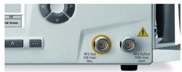
**RF1In/Out** is a 50  $\Omega$  N-type connector (female) on the right-hand side of the front panel.
