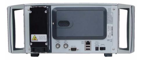
The Stabilock can be equipped with a rechargeable battery module to enable operation in the field, without mains voltage. If you ordered your 2305 with a battery, that battery will have to be installed; see instructions on page 10.
