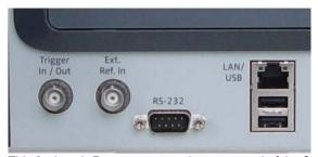
This 9-pin sub-D connector on the rear panel of the Stabilock can be used to control the 9100 remotely via serial interface (RS-232). The command set and the responses conform to the SCPI standard and are explained in the user's guide.
