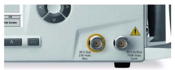
**RF2 OUT** is a 50  $\Omega$  N-type connector (female) on the front panel. It can be used to feed a signal into the receiver section of the unit under test (e.g. a TETRA base station).
