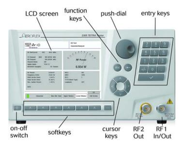
**LCD** The LCD screen shows the menus that guide you through configuration and measurements when the Stabilock is switched on and the operating software is loaded. The menus consist of four different sections:
